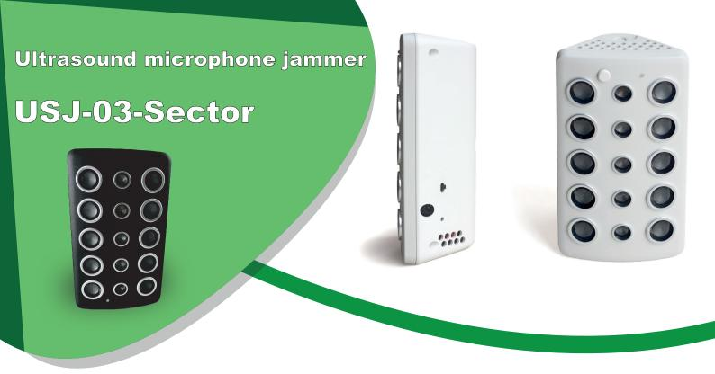
Ultrasound jammer USJ-03-Sector is a powerful device intended to prevent unwanted eavesdropping or making an unauthorised recording using various spy and recording devices, e.g.:
